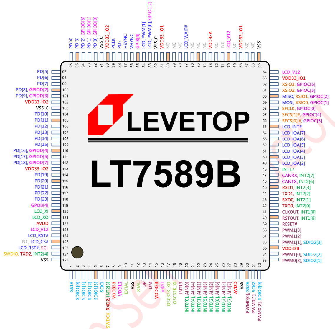
Figure 5-2: LT7589B Pin Assignment (LQFP-128Pin)
