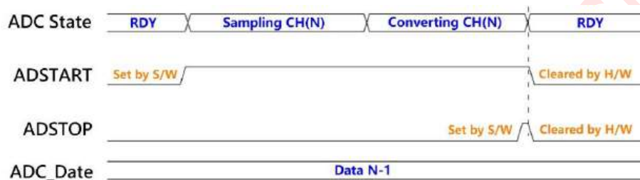
Figure 31-5: Stopping an Ongoing Conversion
